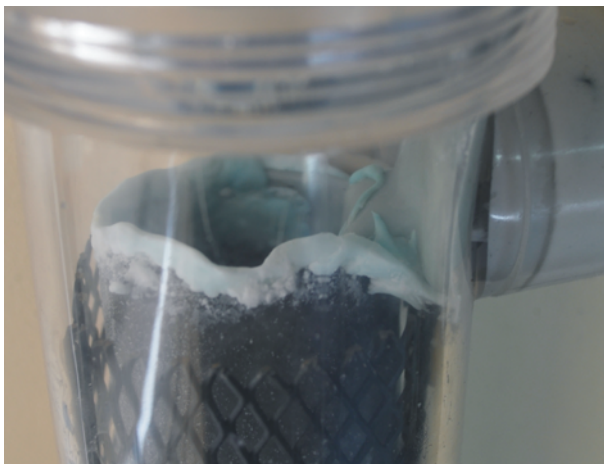
The only localised deposit that formed after 12 months use in this pebble surfaced pool.
